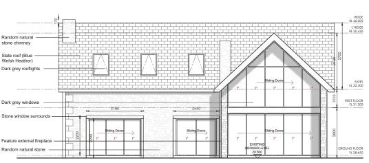
Proposed Elevation - Rear Scale 1:100
